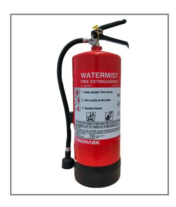
Watermist Extinguishers are suitable for most common types of fire including Class A combustible materials and Class F cooking oil and fat fires. The water mist can also be used on electrical fires up to 1000v.
